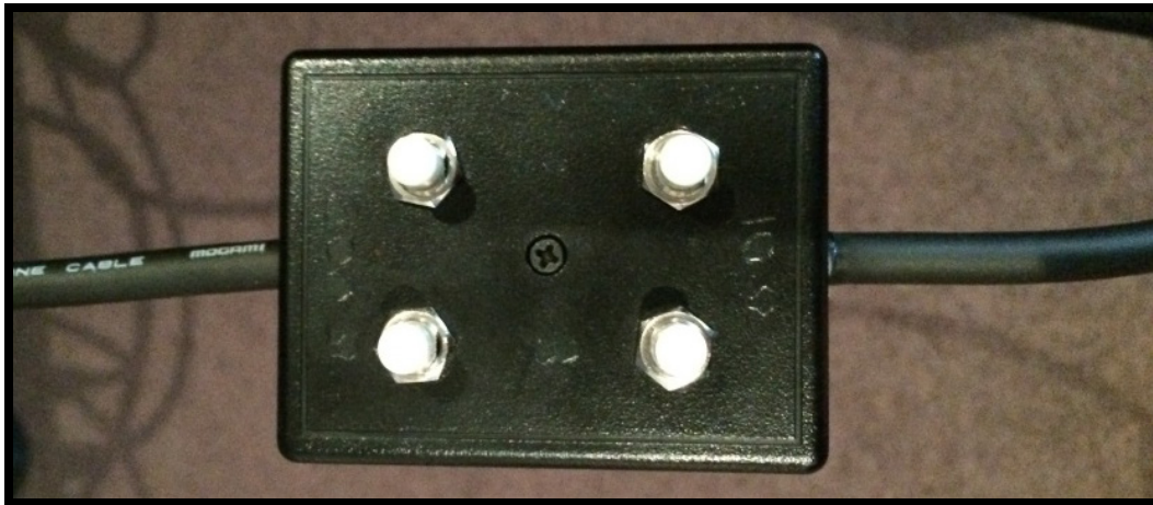
Figure: Box made by Phillip Sztenderowicz to perform CMRR test
