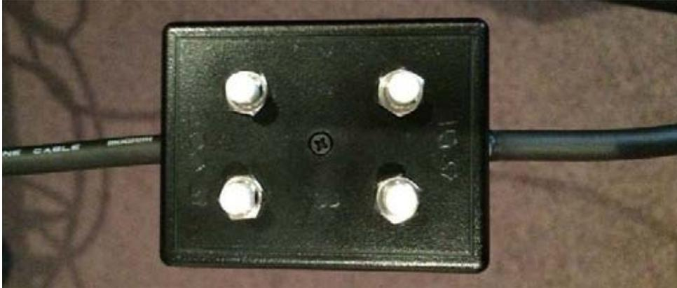
This particular cable is balanced XLR on both ends and allows inserting both 10 Ohm and 600 Ohm resistors in line. However, moving forward only 10 Ohm capabilities are required. To make it as easy as possible for users it would be ideal to have balanced, unbalanced, stereo, and mono versions of this peripheral for sale. In addition to this an open hardware schematic could be drawn and published so that others could make their own or have someone else make it for them.
