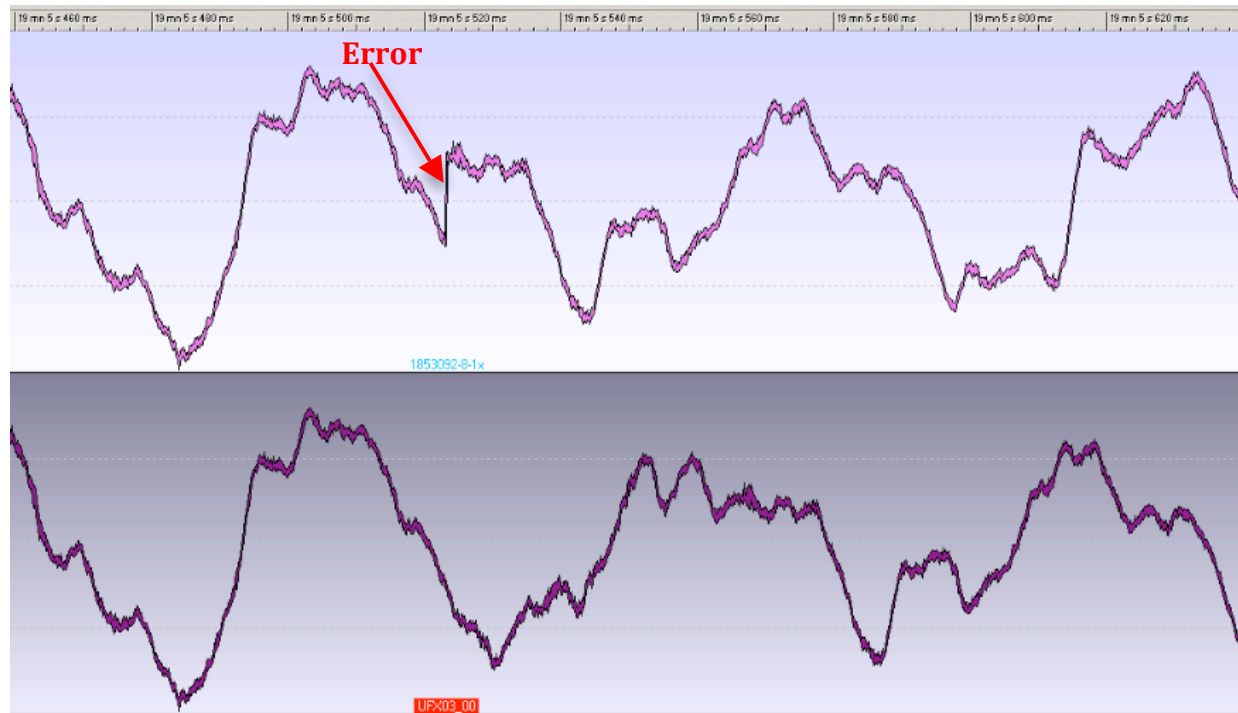
Figure 4: DAW file with interstitial error compared to the intact DDR file
