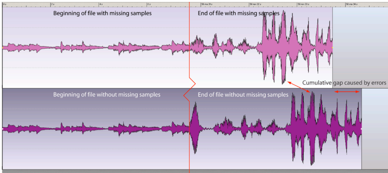
Figure 7: Demonstrating the beginning and end of the DAW and DDR files. Note that they are synchronized in the beginning and that by the end they are out of sync due to missing samples in the DAW file.
